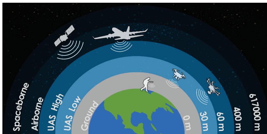
Figure 2. Examples of ground-based, airborne, and space-borne sensors and their typical operational altitudes.
