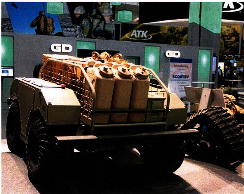
Figure 9. The General Dynamic MUTT can be configured to carry a weapon system or cargo saving on manpower when executing resupply. In the future a simplified pallet loading system with a winch could speed you field loading of prepackaged resupply from airdrops, UAS deliver and ground convoy.
