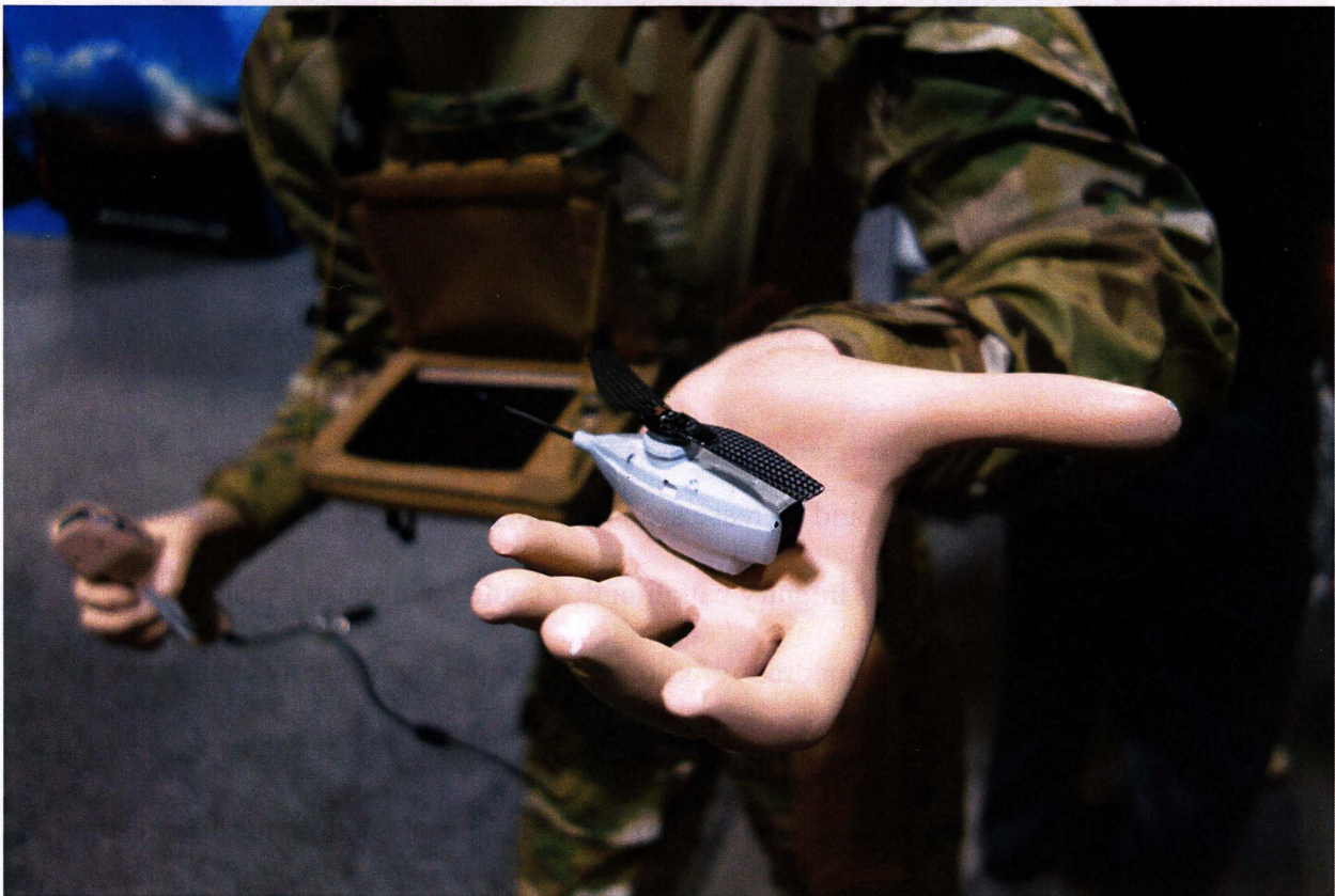
Figure 3. Prox Dynamics' PD-100 Black Hornet is nano UAS technology which has recently entered service with a handful of western armed forces. Weighing only 18 grams (1.3kg per system) and flying at 18Kph, with FLIR, live video and photo feeds over a 1.6km data link it provides a useful combat edge to the operator. Systems like this will have enhanced capability and will be ever present with friends and foes in future conflicts.
