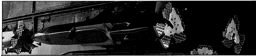
Figure 5: Raytheon's Miniature Air Launched Decoy
