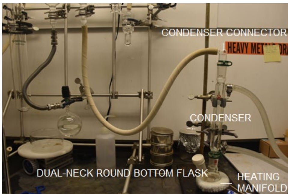
Fig. 4 Solvent reflux reaction under inert gas using a condensor
