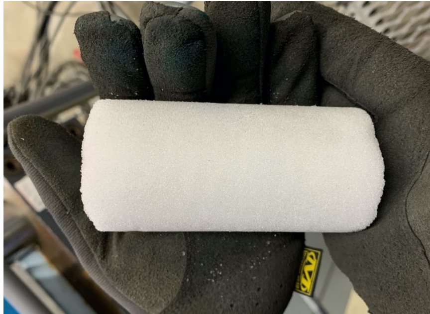
Figure 2. Snow-sample cylinder (133_mx_01) after sintering.
