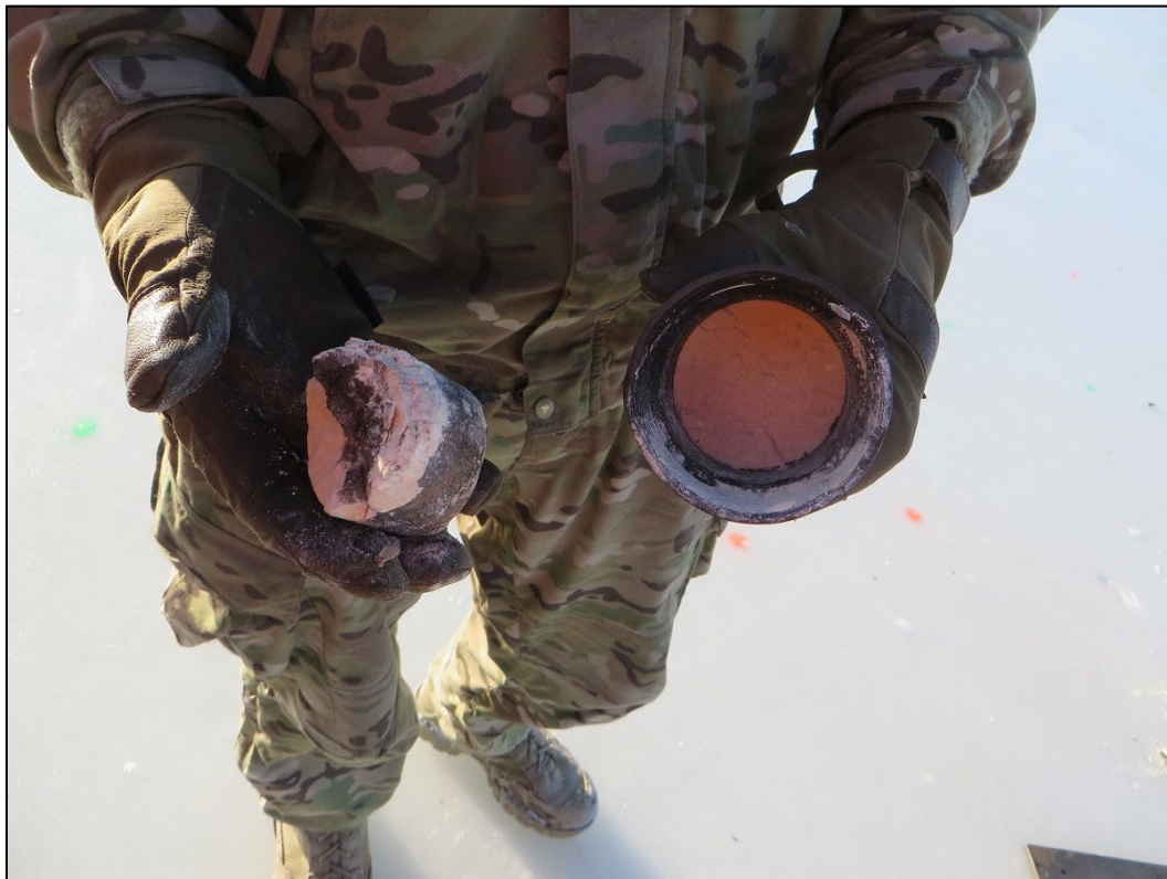
Figure 5. An initiated dud from an attempted LO detonation of an 81 mm Composition B (Comp B) round.
