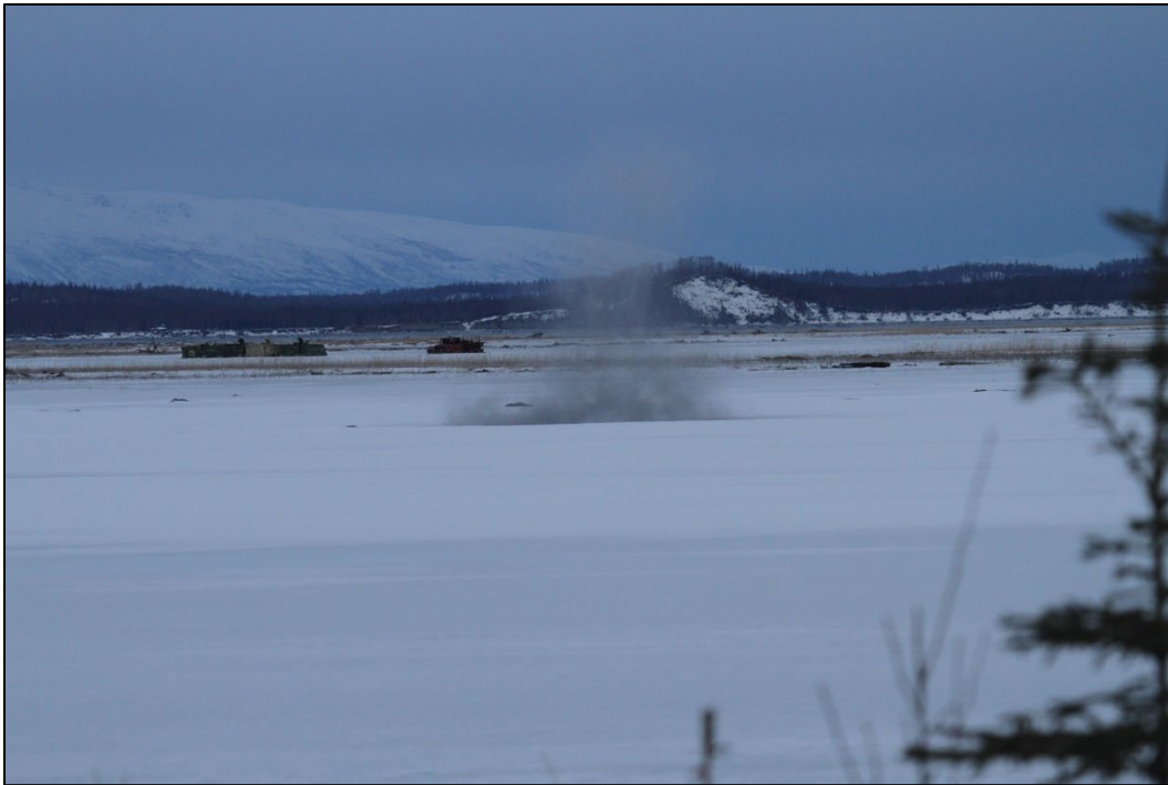
Figure B-3. Example 3 of a depositional and aerial plume immediately following detonation of a 60 mm IMX-104 cartridge from this study using the IMP fuze setting.
