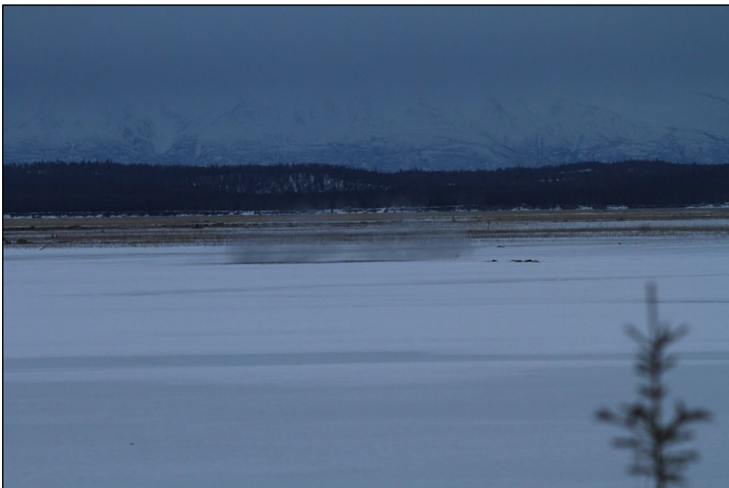
Figure B-2. Example 2 of a depositional and aerial plume immediately following detonation of a 60 mm IMX-104 cartridge from this study using the IMP fuze setting.
