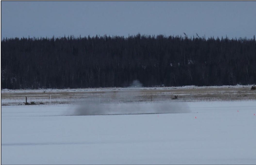
Figure B-1. Example 1 of a depositional and aerial plume immediately following detonation of a 60 mm IMX-104 cartridge from this study using the IMP fuze setting.
