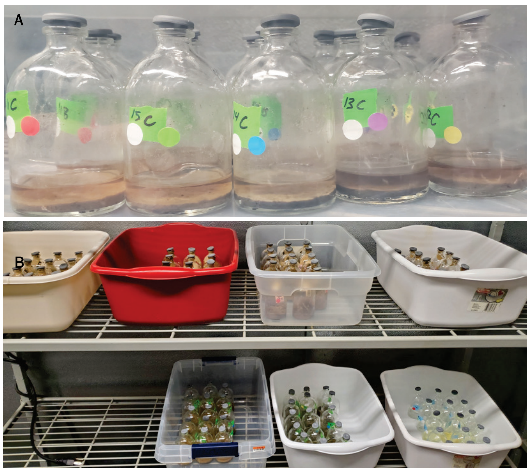
Figure 7. Microcosm setup with A) individual microcosms and B) all the microcosms in a 30°C incubator.
