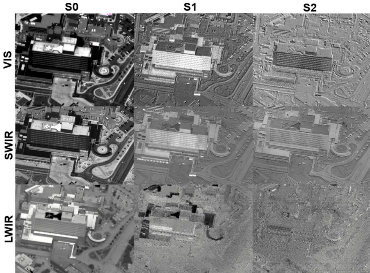
Figure 4. Imagery matrix showing spectropolarimetric (VIS, SWIR and LWIR) imagery, representing three different polarimetric states (S0, S1, and S2). The scene is of St. Mary's Hospital, Grand Junction, CO.
