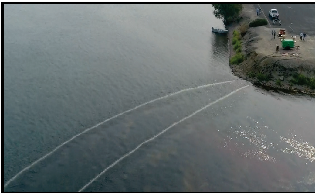
Figure A-2. Bubble curtain in operation at Clover Island Site #5 for Bubble Curtain Evaluation 2. Photo by Terry McNabb.
