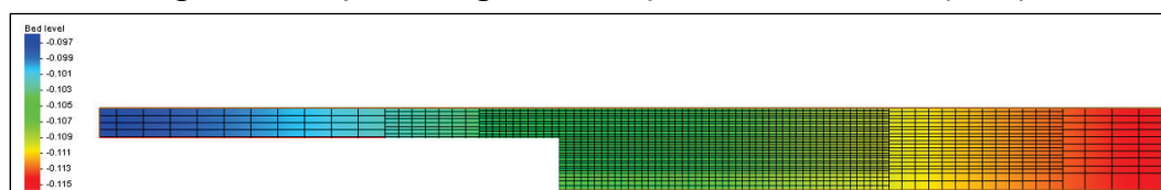
Figure 26. Computational grid for the experimental flume in Xie (1996).
