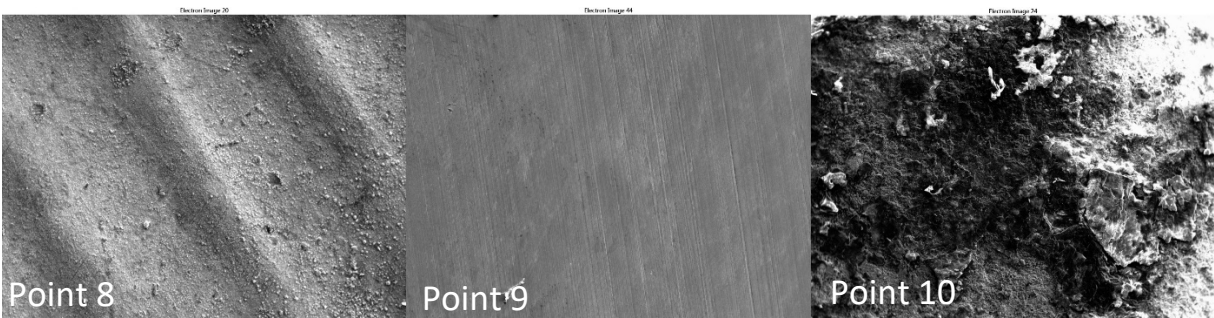
Figure 29: Analysis Points #8 (left), #9 (middle) and #10 (right) SEM Micrograph of Inconel Lid
