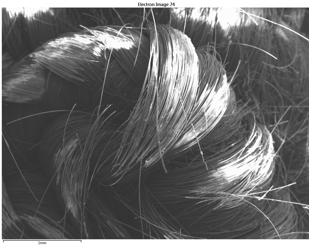
Figure 47: SEM Micrograph of Heat Tape
