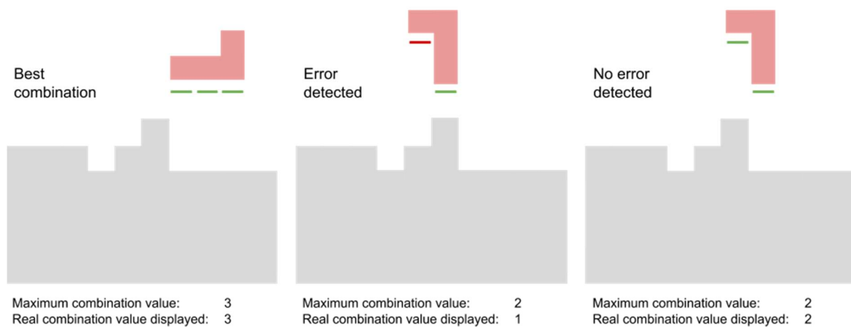
Figure 13. An example of different combinations, computed in background, for the autopilot. The second image represents an incorrect positioning, while in the third image, we see the best combination compared to the one shown in the first image.
