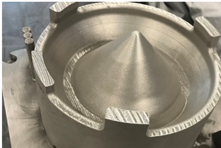
Figure 2: The F110 Additively Manufactured cobalt-chrome sump cover (Davies, 2021).
