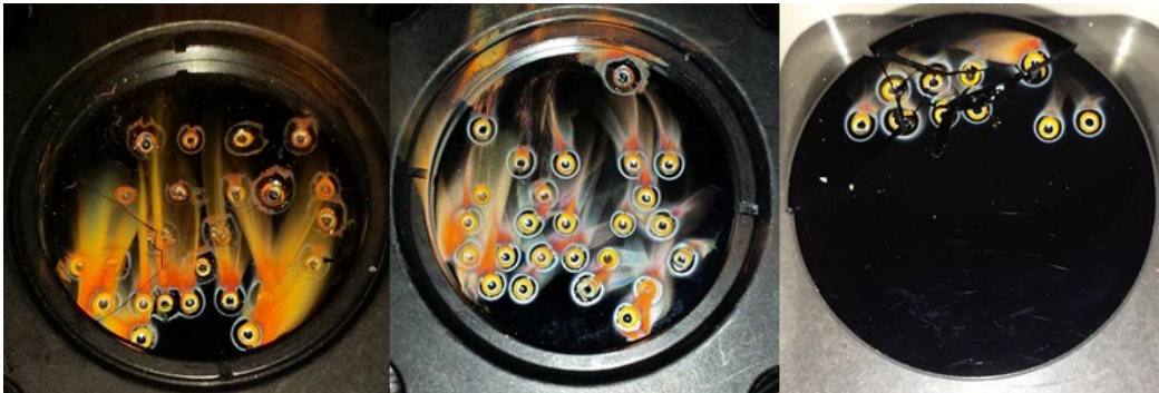
Fig. 12 Front surface of the three IRG-25 test samples after testing. Damage tests start from lower powers at the top left to higher powers at the bottom left, generally.
