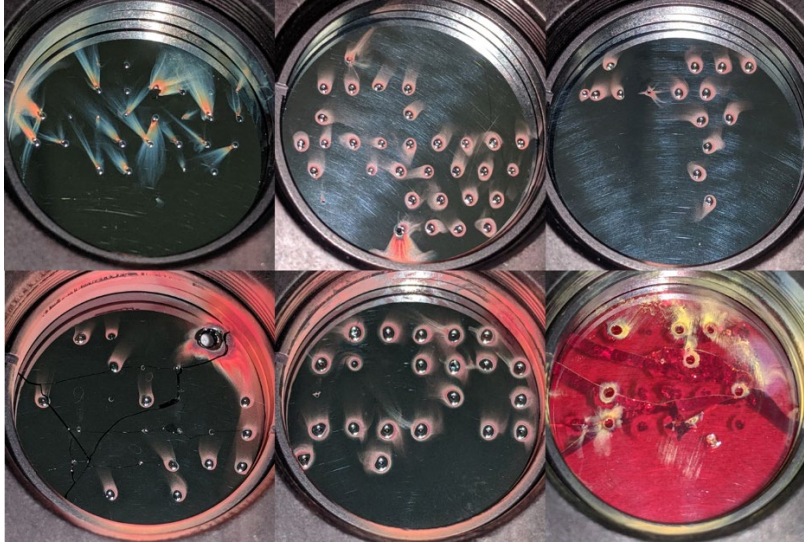
Fig. 43 Back face of the Amorphous Materials Inc ChGs. Top row, left to right: AMTIR-1, AMTIR, 2, and AMTIR-5. Bottom row, left to right: AMTIR-7, AMTIR-4, and AMTIR-6. The As-Se composition ChGs are listed in order of decreasing arsenic.
