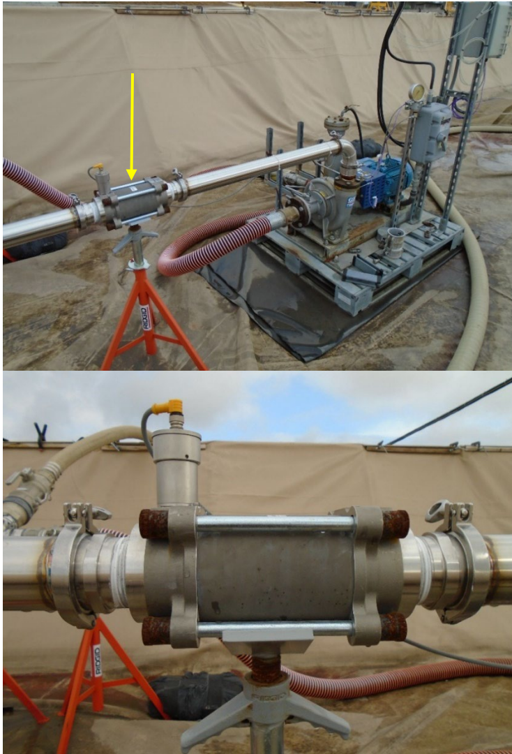
Figure A-1. SwRI Reference Flow Meter #1 (3 inch) Upper Left—Location of Meter Relative to Discharge Side of Pump #1 (Yellow Arrow)
