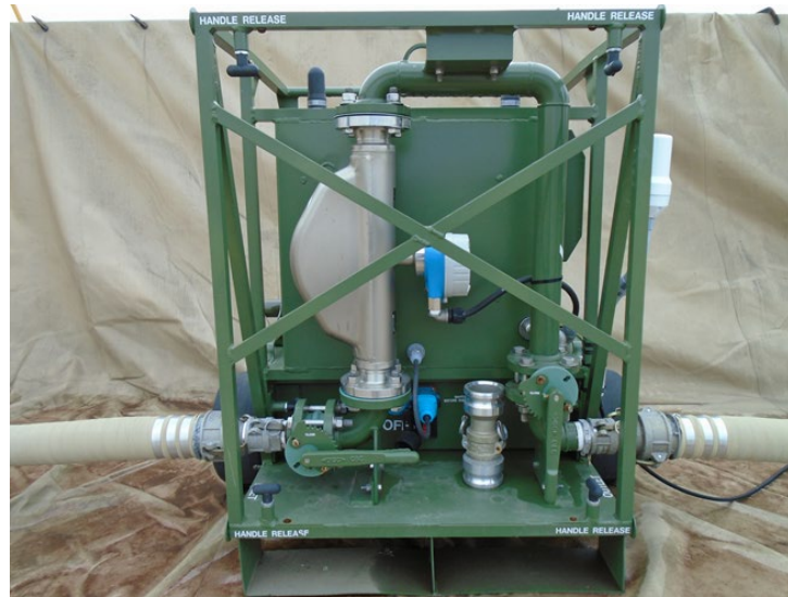
Figure A-11. Candidate Flow Meter #9 (2 inch)
