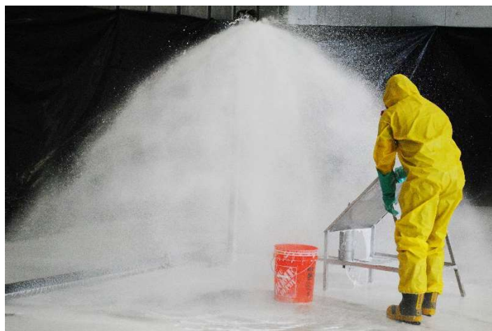
Figure 5. NFPA 11 (3) Foam Collection Device Being Positioned in the Sprinkler Discharge
