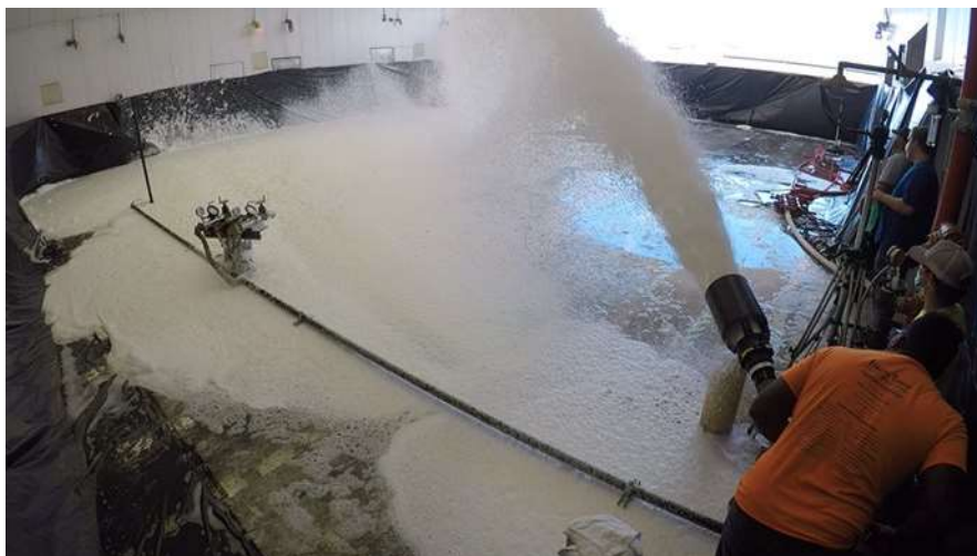
Figure 6. TFT Nozzle Discharge with Air-Aspirated Attachment
