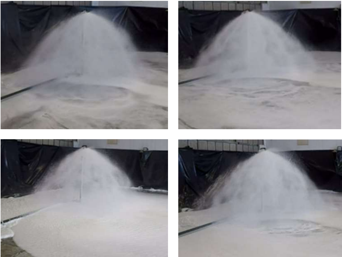
Figure 13. Sprinkler Discharge with all Agents: Solberg (top left), BioEx (top right), Fomtec (bottom left), and National Foam (bottom right)
