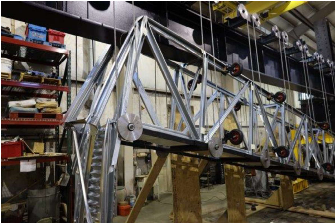
Figure 32: Bending of Tension Chords at Joint Q (AG48-D35)
