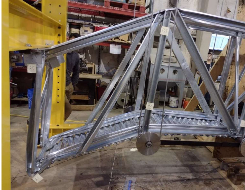
Figure 36: West Quarter of Specimen During Failure (AG48-D35)
