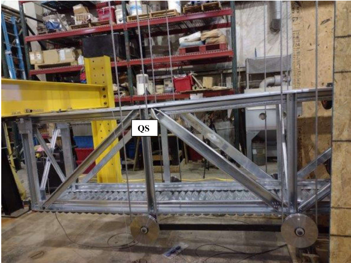
Figure 25: Initial Deformation of Compression Diagonal at Joint QS (AG36-D35)
