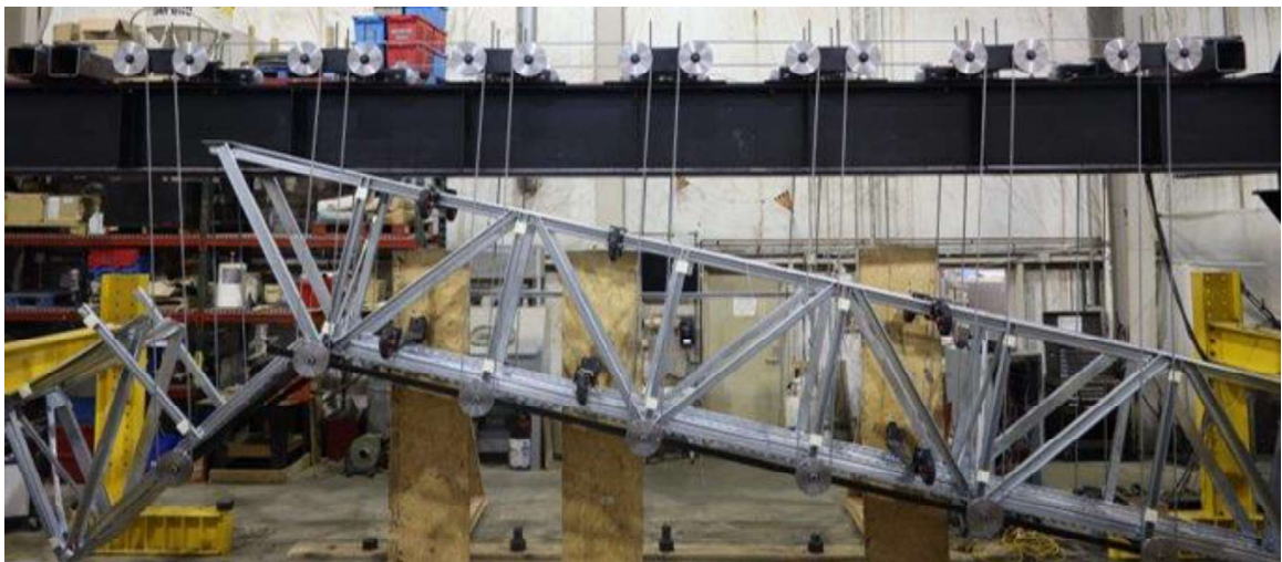
Figure 38: Global Failure of Specimen
