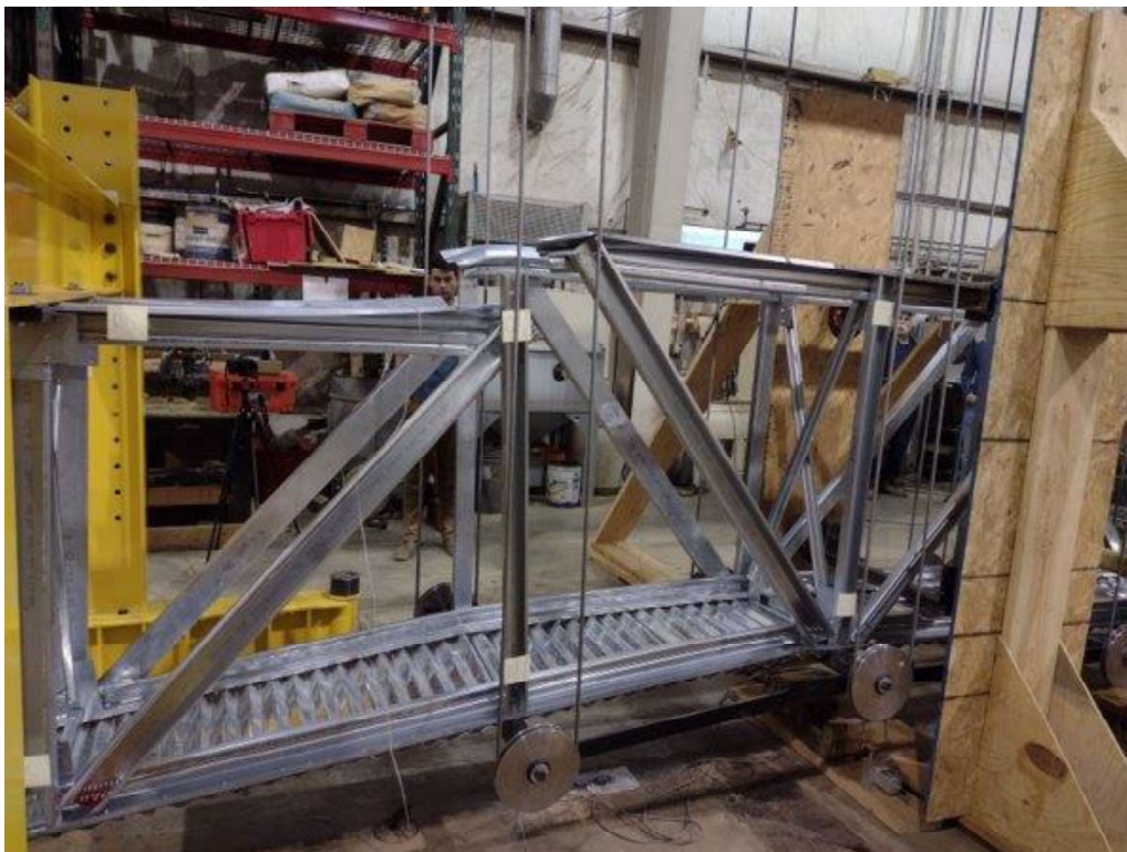
Figure 41: Full Tension Chord Separation
