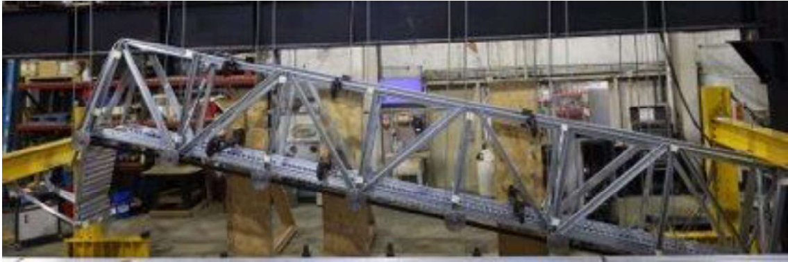
Figure 30: Global Failure of Specimen (AG48-D35)
