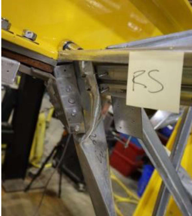
Figure 28: Bearing Connection at Joint RS (AG36-D35)
