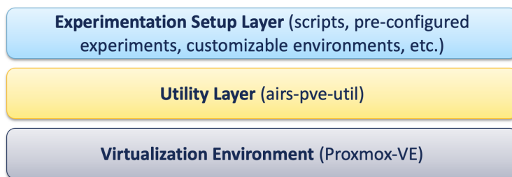
Fig. 1—The underlying virtualization environment provides a foundation for the utility layer, which in turn supports the experimentation setup layer.
