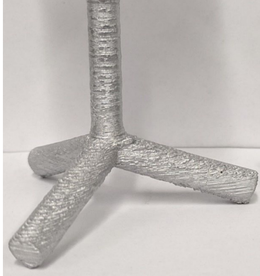
Fig. 4 Tetrahedral cast Al specimen
