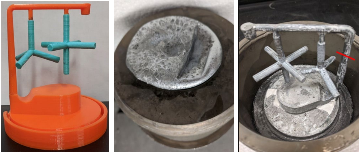
Fig. 1 Photographs of a PLA blank, finished casting, and removed specimens (from casting plaster)
