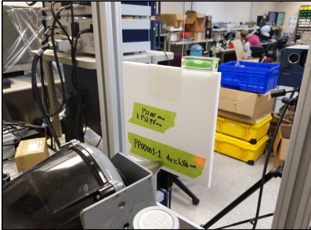
Figure 4.3. Experimental set-up for collecting vibrational eigenfrequencies of thin plate samples. The acoustic excitation source is oriented towards the lower-center side of a PTFE plate, while a Polytec PSV-400 Scanning Laser Vibrometer is aligned for velocity measurements approximately 1 m from the other face.
