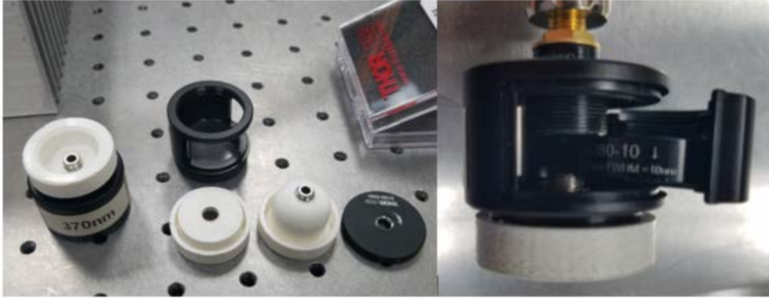
Figure 14. 3D printed optical filter case caps used to narrow fiber to filter gaps.
