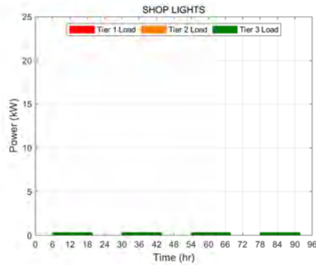
(a) Shop Lights Tiered Electrical Load
