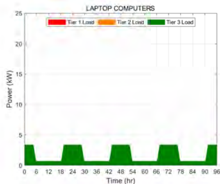
(e) Laptop Computers Tiered Electrical Load
