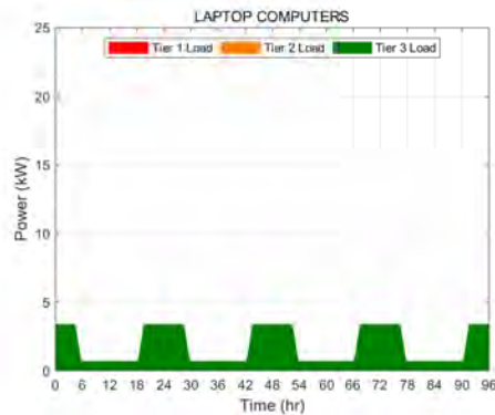
(e) Laptop Computers Tiered Electrical Load
