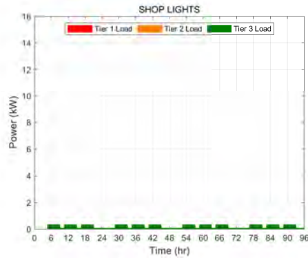
(a) Shop Lights Tiered Electrical Load
