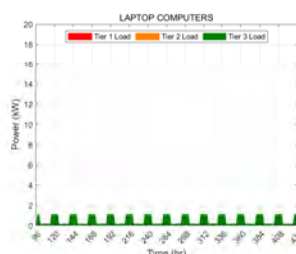
(b) The laptop computers tiered electrical load for the shelter during the simulation epoch of [96–432] h
