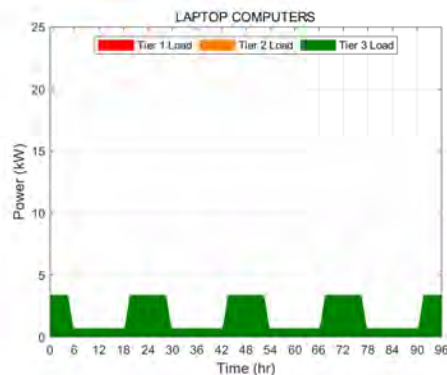
(e) Laptop Computers Tiered Electrical Load
