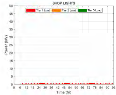
(b) Shop Lights Tiered Electrical Load
