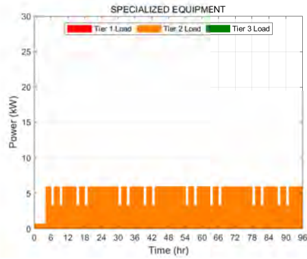
(a) Specialized Equipment Tiered Electrical Load
