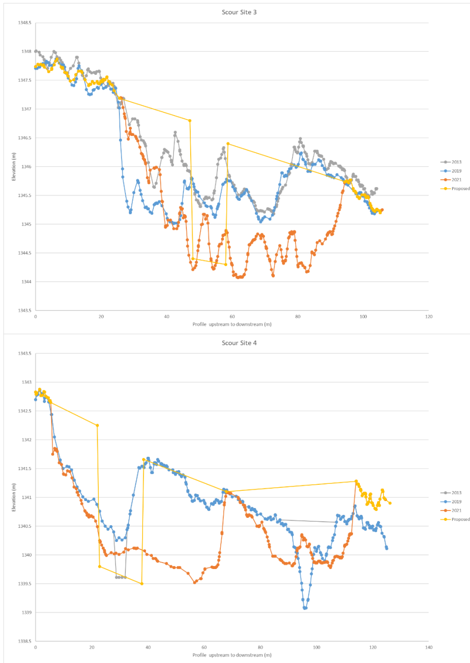
Figure 43. Scour hole shape and size progression from 2013 to 2021, including dimensions of proposed constructed diversion weirs, at scour locations 3 and 4.
