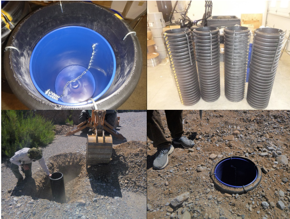
Figure 7. Pit trap samplers and installation.
