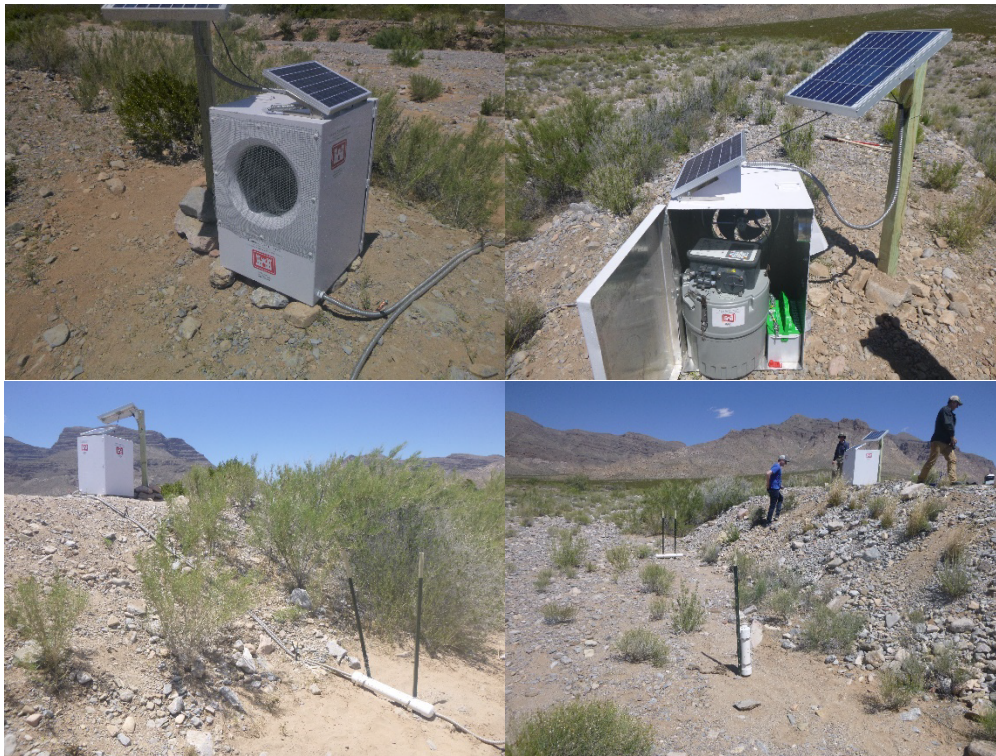
Figure 11. Typical ISCO installation ( top ), typical installation of samples, suction lines, and intakes ( bottom ).
