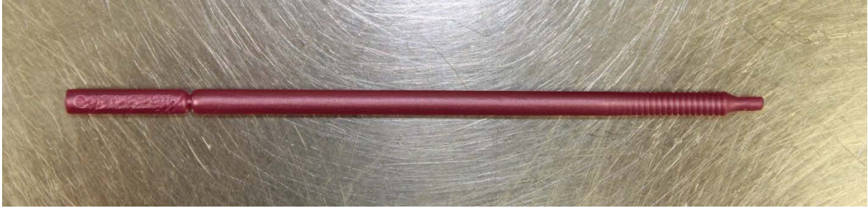
Figure 3-19. Modified microbrush used to adapt the composite within the plastic mounting mold.
