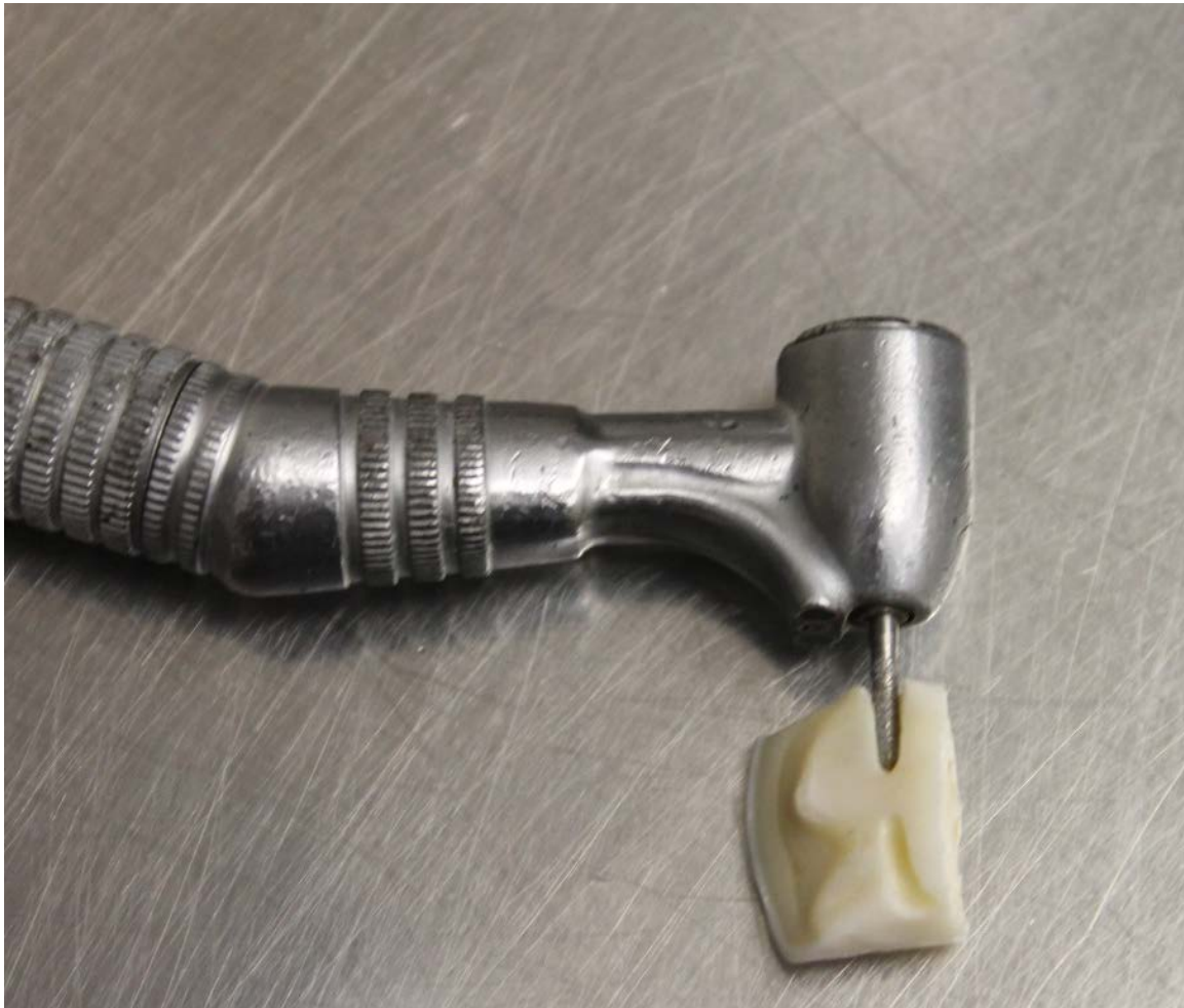
Figure 3-2. Retention cuts placed in the bovine tooth using a high speed handpiece and a tapered diamond bur.
