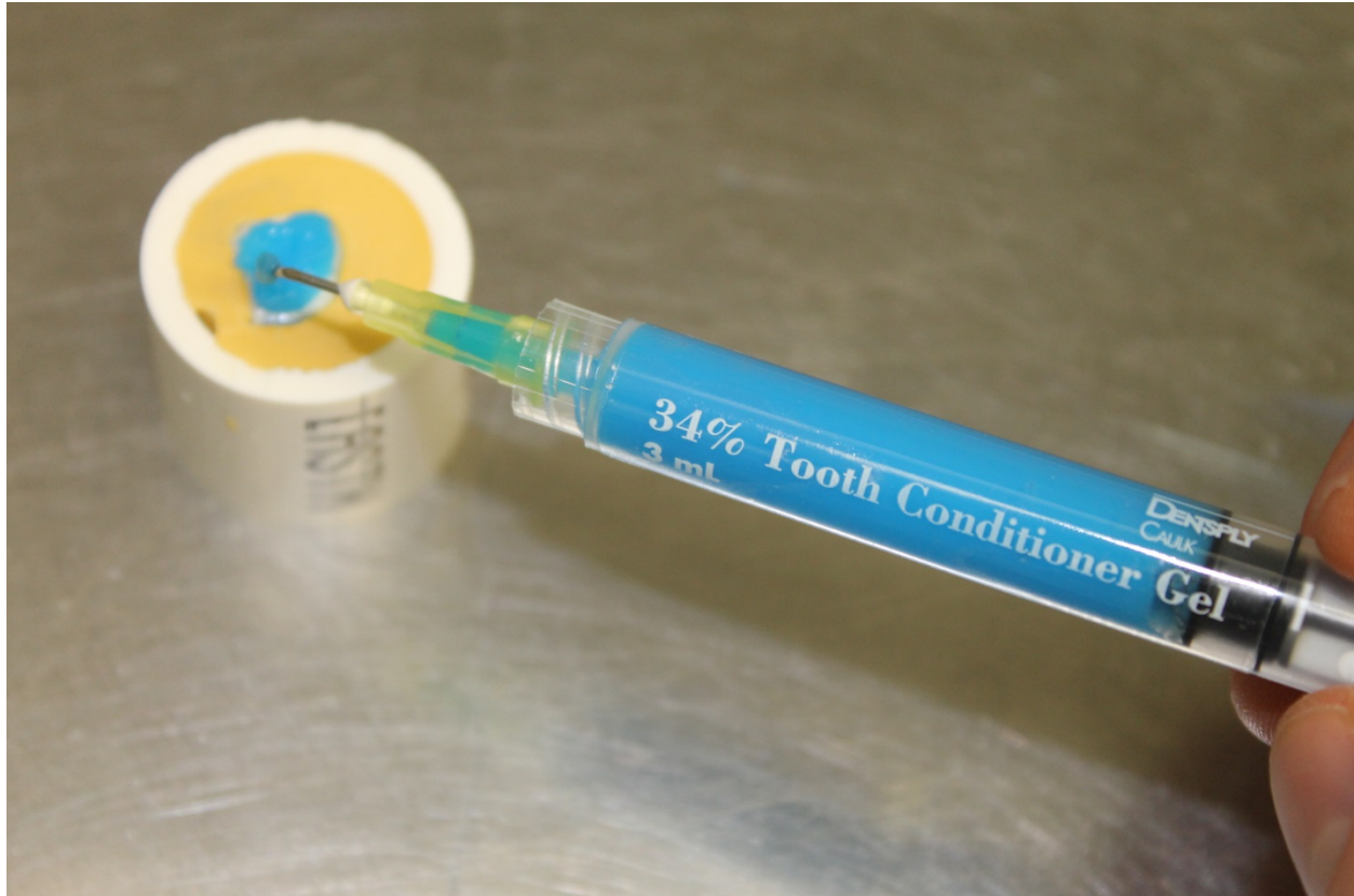
Figure 3-12. Seventy-five teeth had the facial surface of the crown etched using Dentsply (34% Phosphoric Acid) for its designated time.
