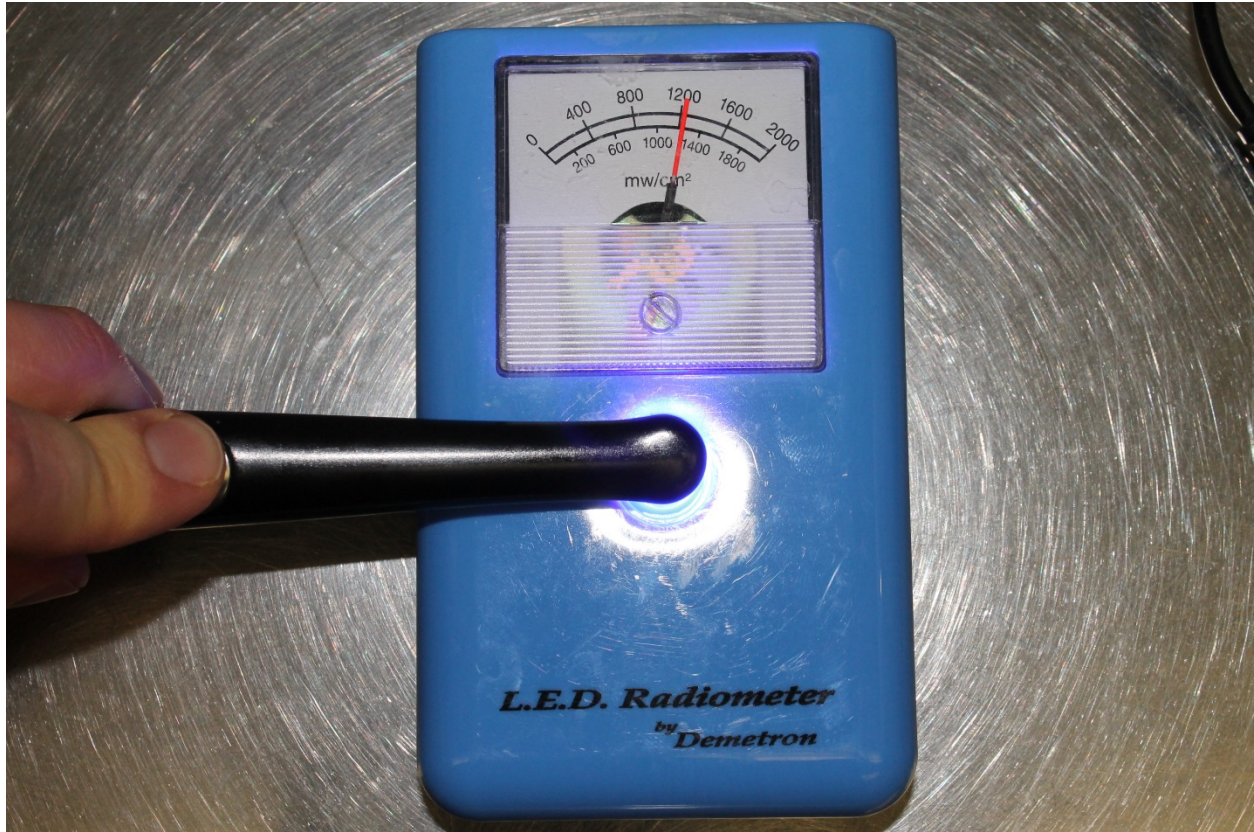
Figure 3-14. Prior to bonding, the curing light was tested using an L.E.D. Radiometer.
