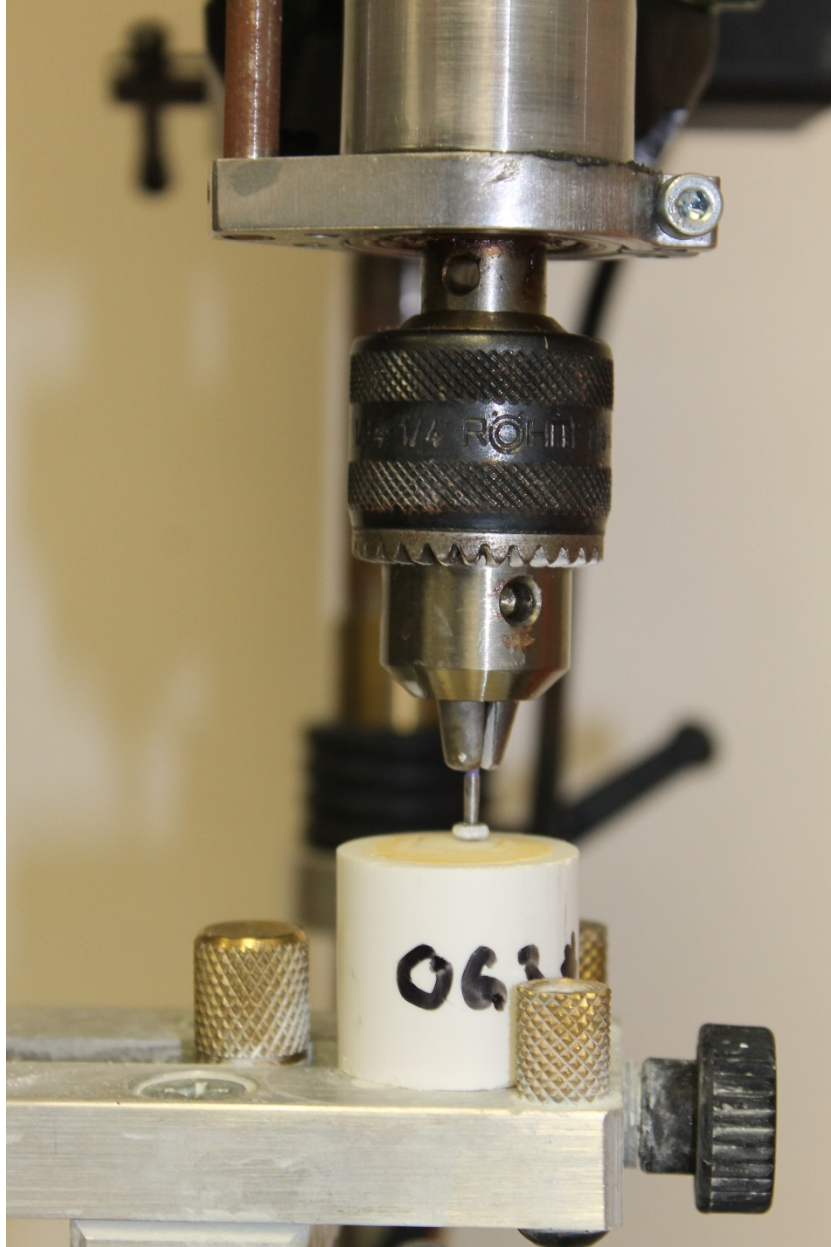
Figure 3-7. The facial surface of the crown was flattened using a drill press and a diamond course bur.
