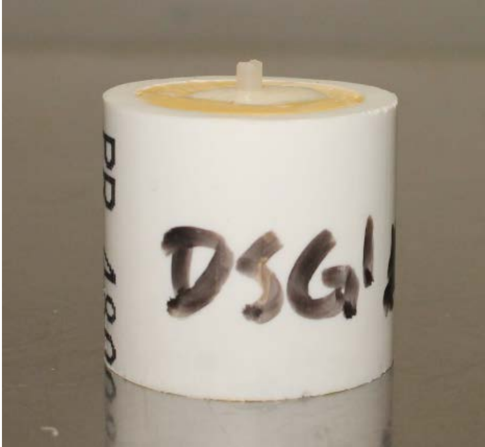
Figure 3-22. Composite resin rod after being removed from the mounting jig. Labeling with a permanent marker was done for each specimen to identify the specimen's subgroup and bonding order.
