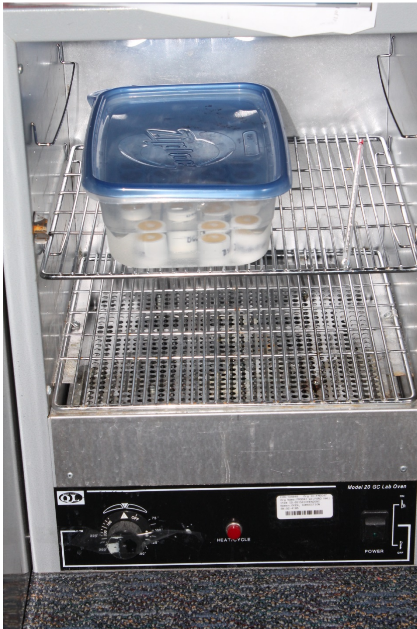
Figure 3-5. Specimens stored at 37 degrees Celsius in a laboratory oven (Model 20GC, Quincy Lab, Chicago, IL).
