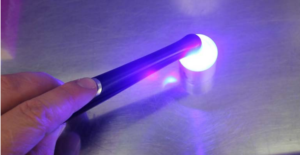
Figure 3-17. A dental curing light was used to cure the primer at maximum intensity for three seconds.
