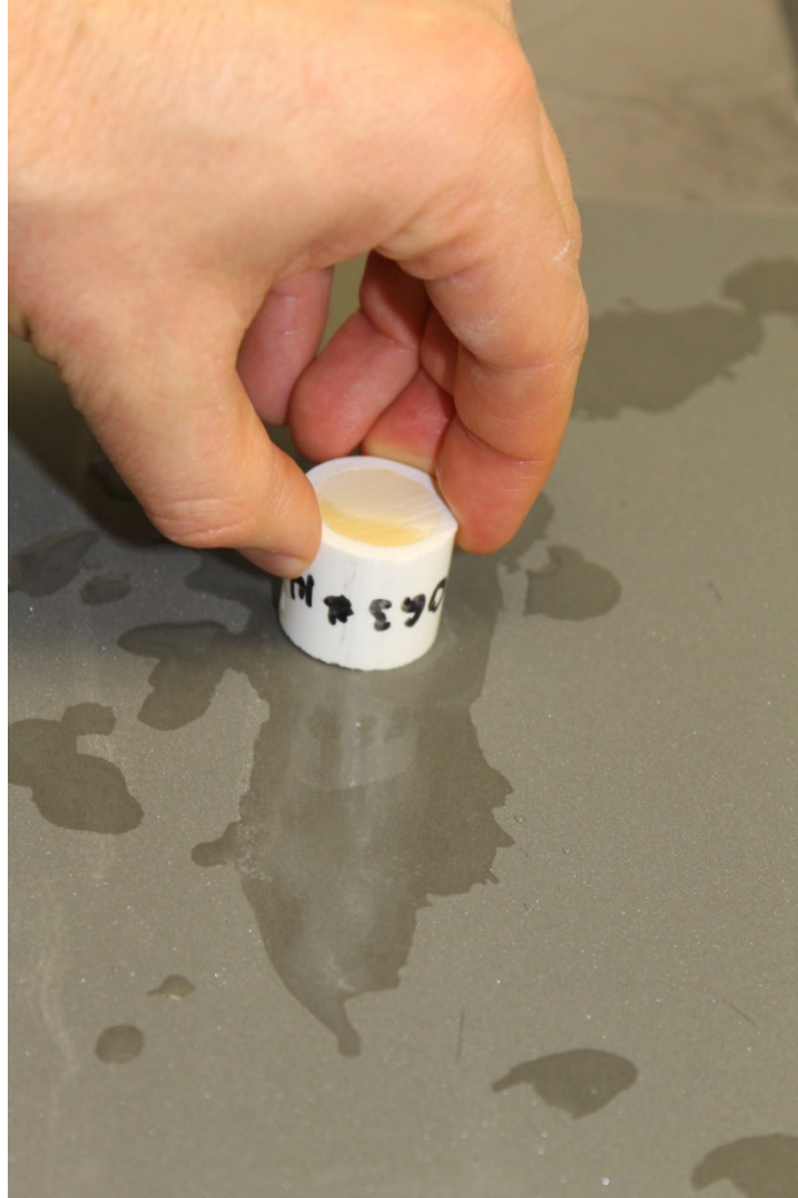
Figure 3-8. Each tooth was sanded flat using 600 grit sandpaper. The specimens were sanded perpendicular to the sandpaper on a flat surface for ten strokes. They were then rotated 90 degrees and sanded in like manner for another ten passes.
