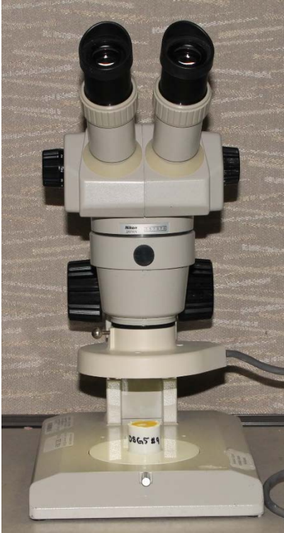
Figure 3-25. Microscope used to evaluate the fracture mode of the resin rods after shear bond strength testing.
