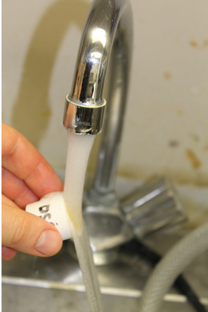
Figure 3-13. After etching, the teeth were then rinsed using a heavy stream of tap water for ten seconds.
