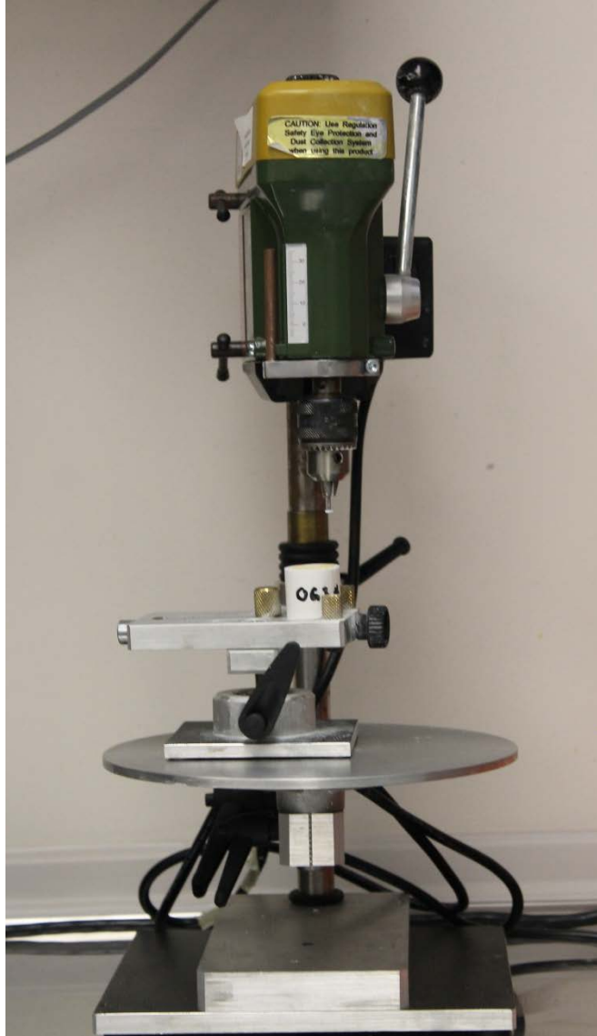
Figure 3-6. The facial surface of the crown was flattened using a drill press (Proxxon TBM 115 Type 38128, Luxemburg) and a diamond course bur.
