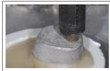
Figure 3: Tooth specimen mounted in universal testing machine with round-ended blade lowered onto marginal ridge in preparation for loading force.
