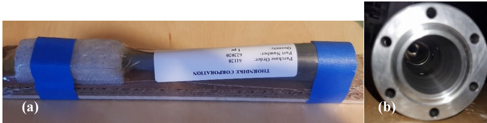
Figure 2.11. Shows (a) the high-power cone load, (b) the load fitted within the experimental assembly.
