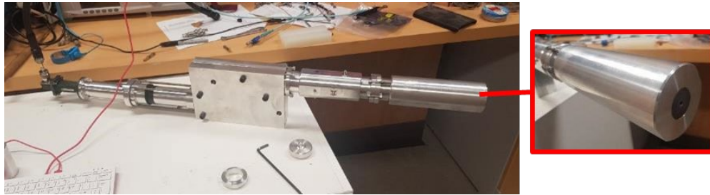
Figure 2.12. Shows the cold-test assembly for characterizing the load termination.
