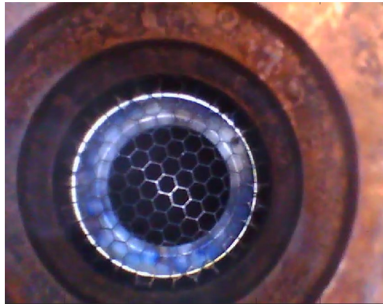
Figure 3.4. Shows the grid and emitter surfaces following characterization of the accelerating diode, photographed in-situ with the SIBWO interaction region attached.
