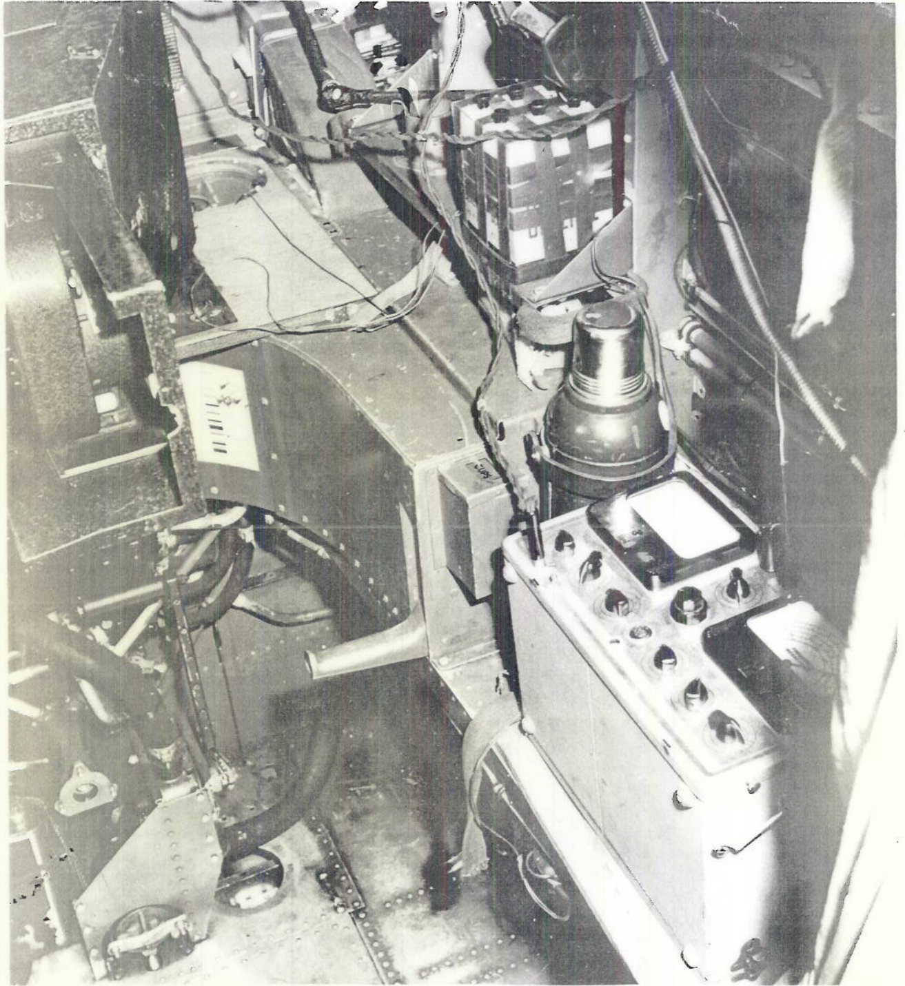
INSTALLATION OF NOISE METER AND PART OF PHOTO-OBSERVER. .
