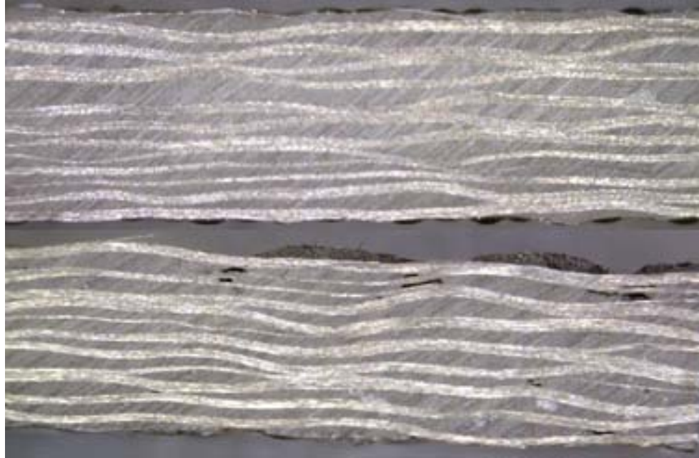
Figure 17. Pre-TOS test optical micrographs for PMR-15/IM7-8HSW-GP (upper) and 0N/ IM7-8HSW-GP (lower) composite cross-sections.
