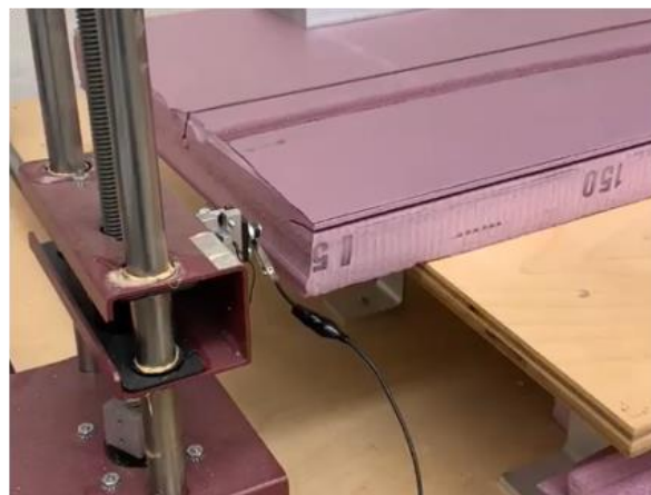
Figure 8. Cutting Wing from Foam
