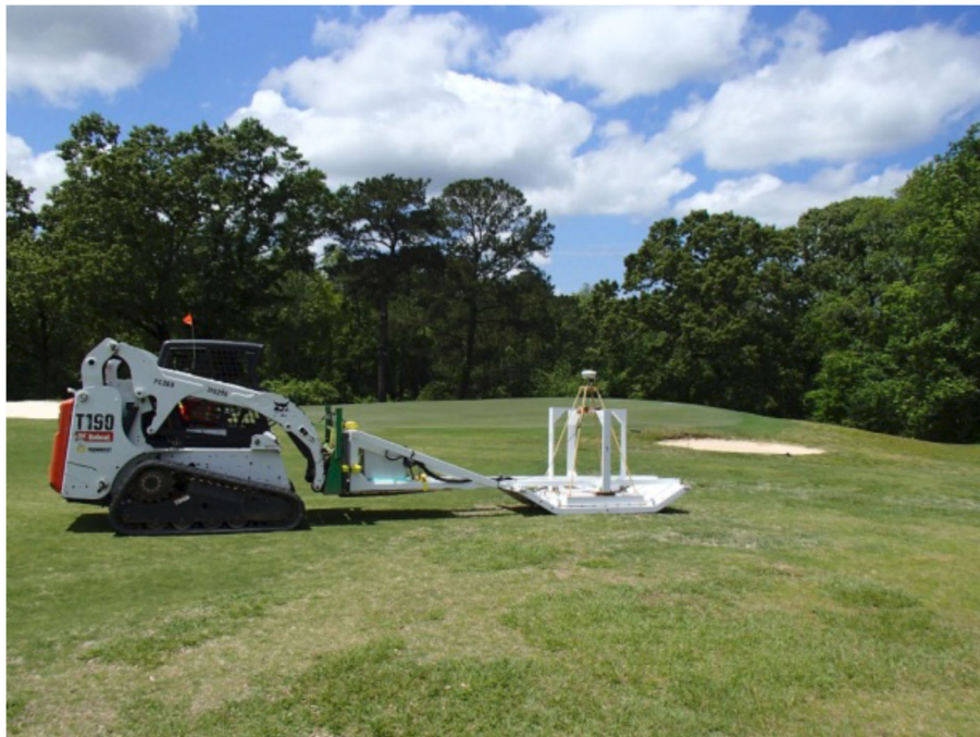
Figure 2. Image of the MetalMapper Classic acquiring data at the Fort Rucker site. Image from Cost and Performance report of ESTCP MR-201161.
