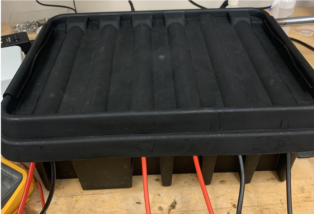
Fig. 12 Weatherized electronics box
