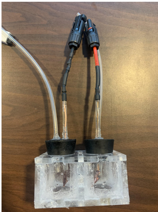
Fig. 8 Assembled H-cell with feedthrough connectors
