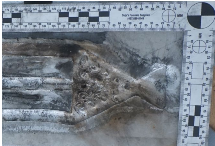
Fig. 11 Experiment 2 perforated triangle cavity
