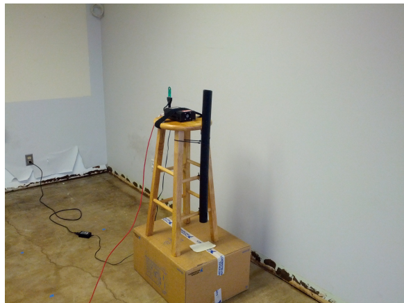
Figure 5: One of the transceivers used to collect UWB impulse response measurements.
