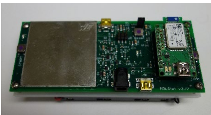
Figure 1. The CStat. The instrument in the photograph is TRL 4. The disposable electrode and its associated cable are not shown. The total weight of the CStat including 6 AA-NiMH rechargeable batteries is less than 300 g with a battery endurance of 20+ hours when running at peak output and a 100% duty cycle.
