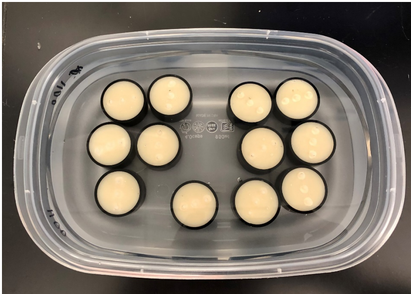
Picture 7: Samples placed in water for 24 hours
