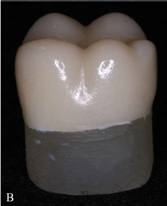
Figure 2: Lithium disilicate (A) and zirconia (B) crowns cemented on NEMA Grade G10 dies.
