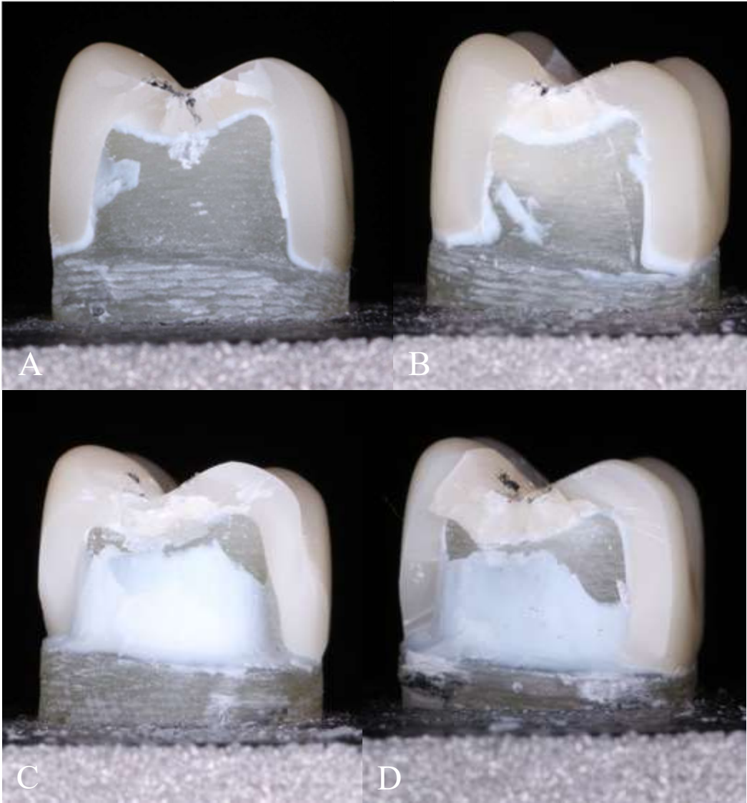
Figure 6: Failed intact (A) and accessed/repared (B) lithium disilicate crowns. Failed intact (C) and accessed/repared (D) zirconia crowns
