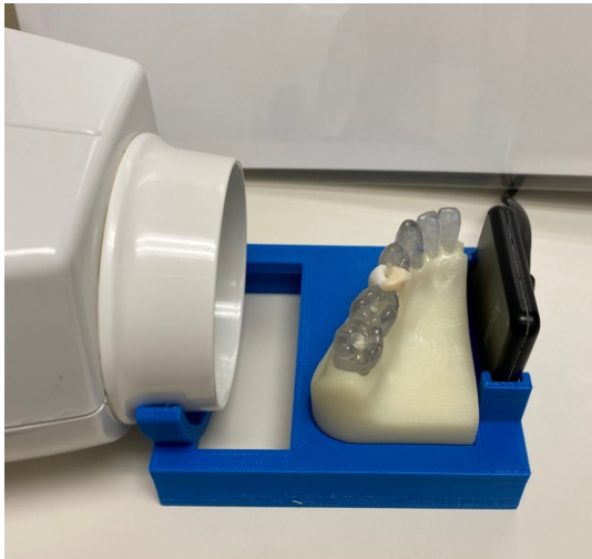
Figure 5: Tooth analog in mandibular left quadrant model placed in jig for standardized radiographic exposure.
