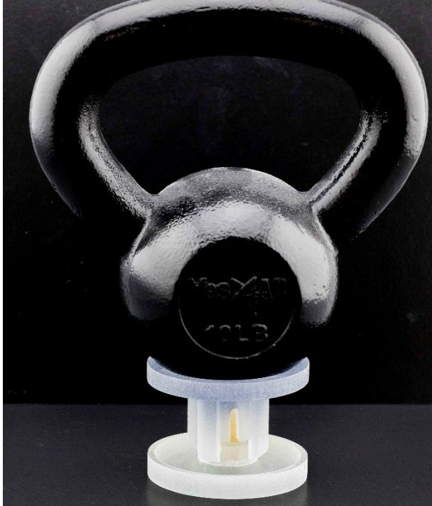
Figure 6. Crown seating index with 10-pound weight
