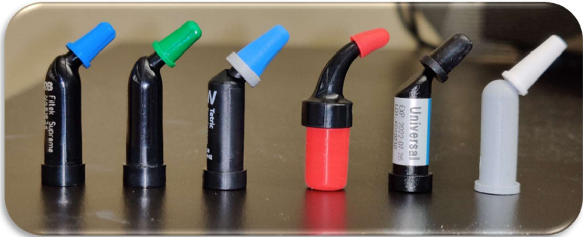
Figure 5. Six RBCs tested from left to right: FSU- Filtek Supreme Ultra, F1B- Filtek One Bulk, TECB- Tetric EvoCeram Bulk Fill, SF3- Sonic Fill 3, VBF- Venus Bulk Fill, & SDR+- Surefill SDR flow plus.
