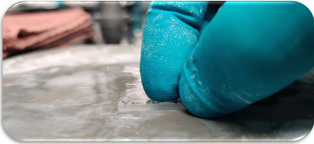
Figure 3. Specimen ground with silicon carbide paper to remove protruding edges.
