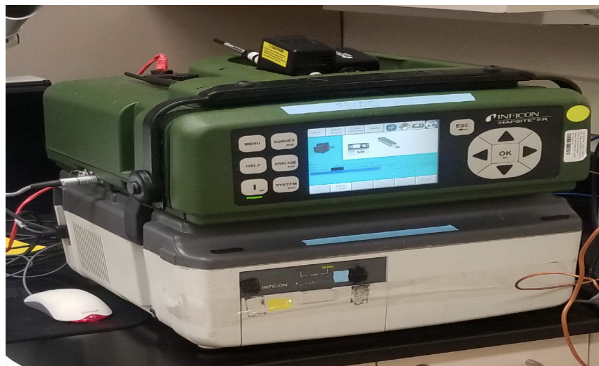
Figure 3.1. HAPSITE® ER configuration with the service module and the SPME sampling system.
