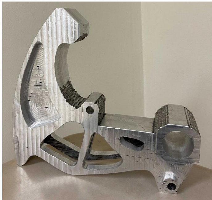
Figure 27 Topology optimized bellcrank produced by hWAAM
