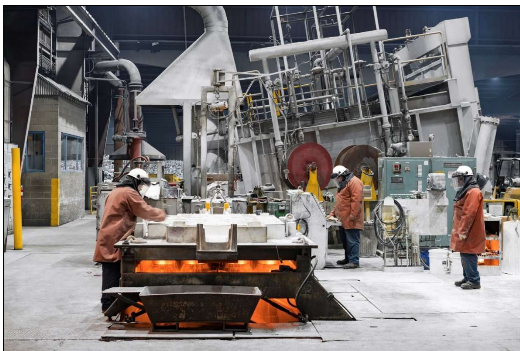
Figure 1: Aluminum Casting Process, Norsk Hydro
