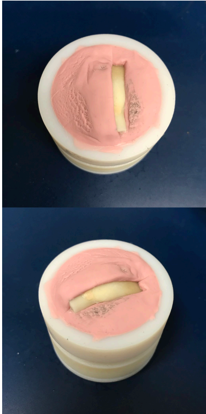
Figure 4. Embedding and protection of one-half facial surface. Lab putty was used to embed the specimen in the toothbrushing well with the left side of the facial surface protected from TBS.
