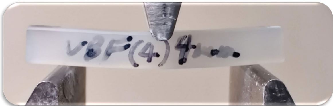
Figure 6. Specimen subjected to flexural strength testing using the MTS Systems Corp Alliance RT/5 testing machine
