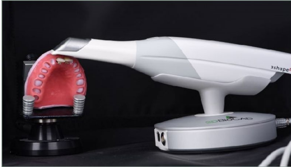
Figure 2. Experimental device set up. The scanner wand was fixed and positioned 5 mm from shade tab surface to scanner tip. To maintain constant distance during scans, gingival matrix positioned on dental survey table. Only survey table moved during scanning
