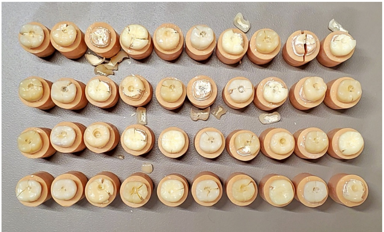
Figure 6. Fracture patterns of all crown materials tested.
