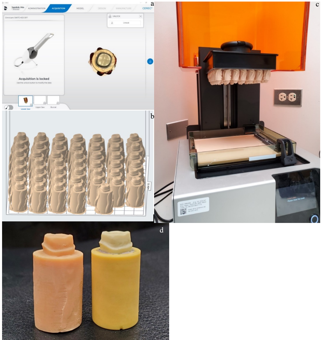
Figure 1. a-c: Digital workflow to fabricate SLA (3-D printed) dies; d: SLA and Master dies.
