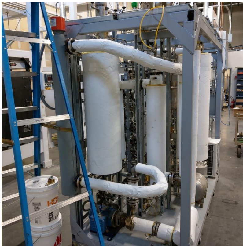
Figure 2. Image of the assembled 2-stage RWGS/FT pilot-scale reactor skid
