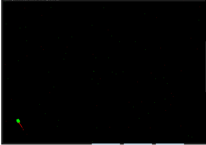
Figure 19: An example of the EBC’s pixels taking time to settle after an RSO passes, visible as the red trail behind the RSO.
