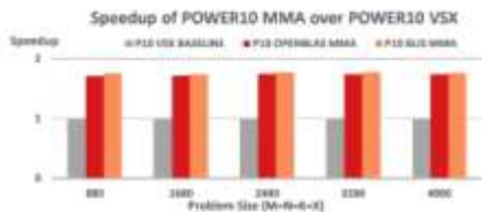
Fig. 1: Performance of double-precision BLIS and OpenBLAS POWER10 MMA kernels over a baseline POWER10 VSX for square problem sizes. From the plot, we see that POWER10 MMA achieves 1.73-1.76 \times speedup (out of a theoretical achievable speedup of 2 \times ) over POWER10 VSX implementation.
